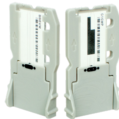
Figure 1: Flow cell from the standard kit (left) and micro kit (right)
