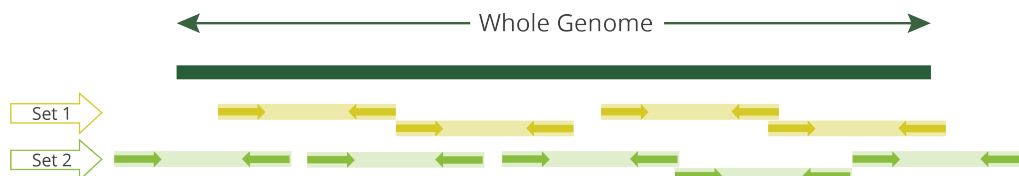
Figure 2 Tiled amplicons for complete coverage
